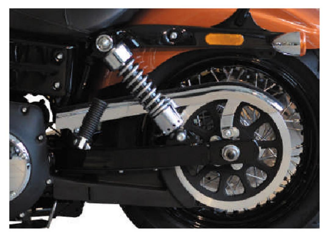
The devil is, as always, in the details: Some models have fender-strut-covers. Those are covering the gap to the fender. Here it is necessary to loosen the strut-cover and to put the included plastic washers between the cover and the struts to both retaining bolts. So the gap between cover and fender is getting bigger, which allows threading the strap easily through.
