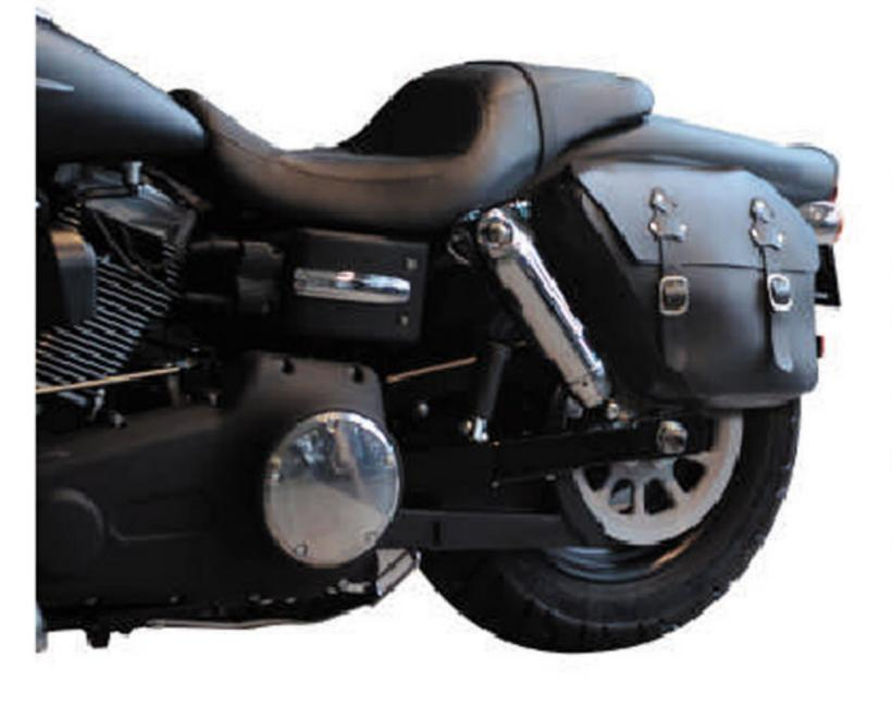
Well, that looks great! Now you can load the saddlebag ad libitum. Check periodically, if the bag fits firmly. Through wetness, the leather straps will give in, in the beginning and should then be retightened. Check always that the bag does not get into contact with the pulley or break equipment.
