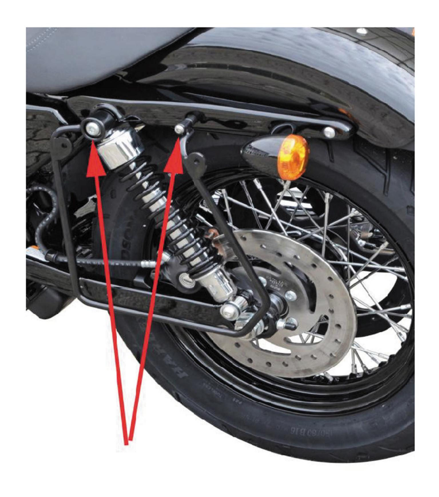
The saddlebag bracket is mounted with 2 screws. The front bolting is done with the shock. For the rear mounting, the serial bolting with the fender struts has to be removed. For the mounting bushings and mounting material is included in the delivery.
