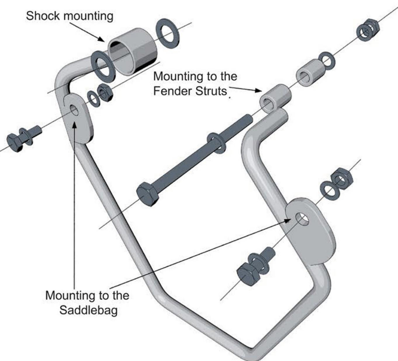
The saddlebag bracket is mounted with 2 screws. The front is mounted with the shock. Please use here the original screws and the two 13x24mm washers. Remove the original screws of the struts. Bushings and mounting material is included to mount the rear part of the bracket. The scope of supply includes screws with different length.
