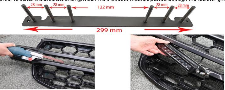
Adjustments may need to be made to the grille to ensure the brackets are securely in place.
