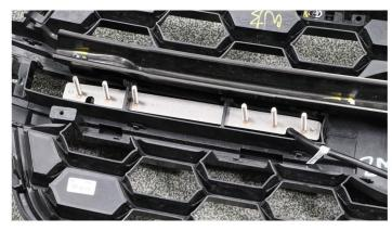
Place a washer on the thread and then the nuts and tighten them with a wrench. Make sure that the bracket does not slip.
